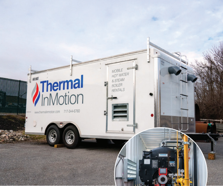
A Burnham boiler inside a Thermal InMotion trailer
